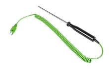
316 Stainless Steel Penetration Probe with a pointed tip for liquid and semi-solid temperature measurement. Comprising of a handle, 2 metre coiled cable and a mini plug.
