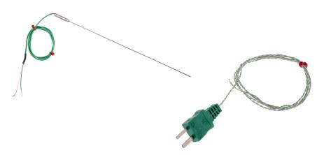
The ideal immersion depth can be achieved in practice by moving the probe into or out of the process medium incrementally; with each adjustment, note any apparent change in indicated temperature. The correct depth will result in no change in indicated temperature.
