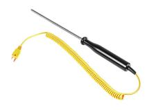
Mineral Insulated Immersion Probe with a rounded tip suitable for semi solid and liquid temperature measurement. Comprising of a handle, 2 metre coiled cable and Type K mini plug. A semi flexible construction allows the probe to be bent or shaped for hard to reach applications. They are suitable for use in corrosive material tests and high temperature molten metal measurements.
