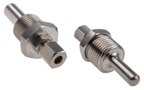
Stainless steel thermopockets of numerous sizes, designed for use with industrial style temperature probes to provide protection for the sheathing from corrosive media, and to facilitate probe replacement without disturbing the process.
